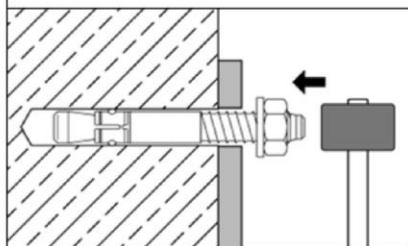
Drive in anchor, such that  $h_{ef}$  or  $h_{ef,red}$  is met. This is ensured, if the thickness of fixture is not greater than the maximum thickness of fixture marked on the anchor in accordance with Annex A2 and A3.
