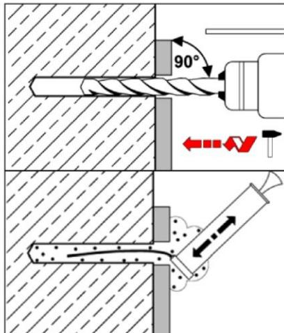
Drill hole perpendicular to concrete surface, positioning of the drill holes without damaging the reinforcement.
