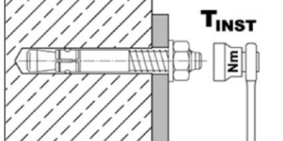
Apply installation torque  $T_{inst}$  as specified in Table B2.
