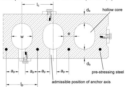
Minimum spacing and edge distance of anchors and distance between anchor groups in precast pre-stressed hollow core slabs
