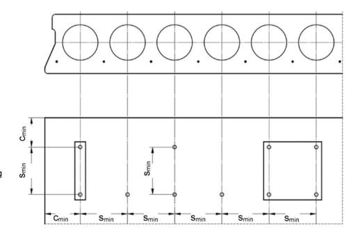
Minimum edge distance  $c_{min} \ge 150 \text{ mm}$
