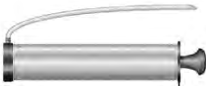
Blow-out pump (volume 750ml) Drill bit diameter ( d_0 ): 10 mm to 20 mm Bore hole depth h_0 \leq 10 d_{nom} see annex B4
