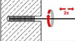
Check brush diameter (Table B4). Brush the hole with an appropriate sized wire brush  $\geq d_{b,min}$  (Table B4) a minimum of **two** times. If the bore hole ground is not reached with the brush, an appropriate brush extension must be used.
