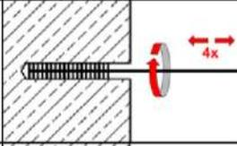
Check brush diameter (Table B4). Brush the hole with an appropriate sized wire brush  $\geq d_{b,min}$  (Table B4) a minimum of **four** times. If the bore hole ground is not reached with the brush, an appropriate brush extension must be used.
