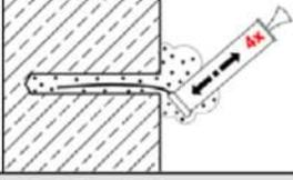
Starting from the bottom or back of the bore hole blow out the hole again a minimum of **four** times.
