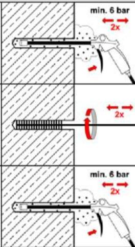
Starting from the bottom or back of the bore hole, blow out the hole with compressed air (min. 6 bar) a minimum of **two** times until return air stream is free of noticeable dust. If the bore hole ground is not reached, an extension must be used.
