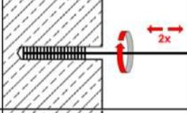
Check brush diameter (Table B4). Brush the hole with an appropriate sized wire brush  $\geq d_{b,min}$  (Table B4) a minimum of **two** times.
