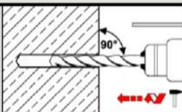
Drill with hammer drill or compressed air drill or vacuum drill a hole into the base material to the size required by the selected anchor (Table B1, B2 or B3). In case of aborted drill hole, the drill hole shall be filled with mortar.
