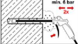
Starting from the bottom or back of the bore hole, blow out the hole with compressed air (min. 6 bar) again a minimum of **two** times until return air stream is free of noticeable dust. If the bore hole ground is not reached, an extension must be used.
