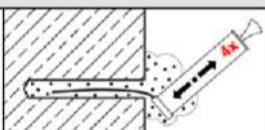
Starting from the bottom or back of the bore hole, blow out the hole with the blow-out pump a minimum of **four** times.
