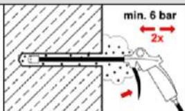
Starting from the bottom or back of the bore hole, blow out the hole with compressed air (min. 6 bar) a minimum of **two** times until return air stream is free of noticeable dust.
