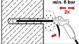
Starting from the bottom or back of the bore hole, blow out the hole with compressed air (min. 6 bar) again a minimum of **two** times until return air stream is free of noticeable dust. If the bore hole ground is not reached, an extension must be used.
