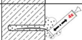
Starting from the bottom or back of the bore hole blow out the hole again a minimum of **four** times.
