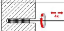
Check brush diameter (Table B4). Brush the hole with an appropriate sized wire brush  $\geq d_{b,min}$  (Table B4) a minimum of **four** times.
