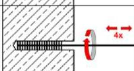
Check brush diameter (Table B4). Brush the hole with an appropriate sized wire brush  $\geq d_{b,min}$  (Table B4) a minimum of **four** times.
