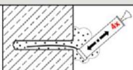
Starting from the bottom or back of the bore hole, blow out the hole with the blow-out pump a minimum of **four** times.
