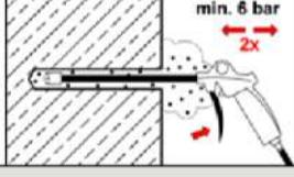
Starting from the bottom or back of the bore hole, blow out the hole with compressed air (min. 6 bar) again a minimum of **two** times until return air stream is free of noticeable dust. If the bore hole ground is not reached, an extension must be used.
