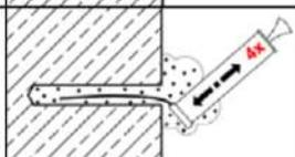
Starting from the bottom or back of the bore hole blow out the hole again a minimum of **four** times.
