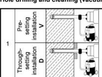
Drill hole perpendicular to concrete surface by using a vacuum drill bit (see Annex B1).
