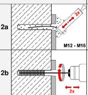
Blow out drill hole from the bottom using Blow-out Pump at least two times.
