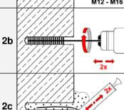
Check diameter of Cleaning Brush. If brush can be pushed into the drill hole without any resistance, it must be replaced. Chuck brush into drill machine. Turn on drill machine. Brush drill hole back and forth along the entire drill hole depth at least **two times** while rotated by drill machine.
